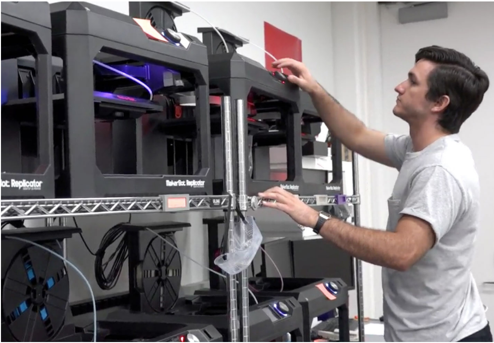
Florida Polytechnic University laboratory technician Samuel de Oliveira uses a 3D printer to produce components for face shields. Image courtesy of Florida Polytechnic University.
