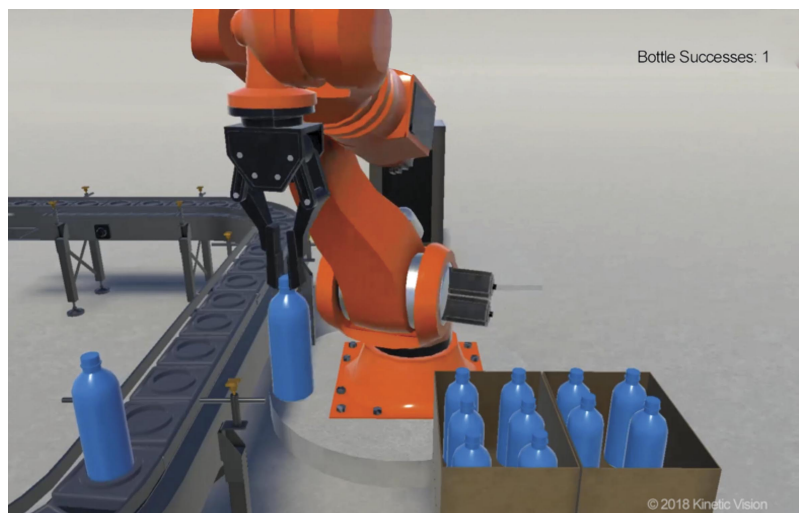
Figure 5: Still-frame from pick-and-place robot interactive VR simulation.
