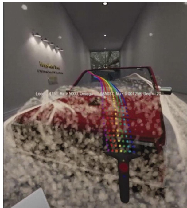
Figure 4: Coloured streak-lines injected into the flow by the user through the VR motion controllers.
