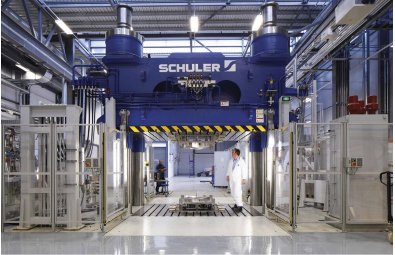
Figure 4: Europe's only open-access 3.4m x2.6m press installed and making parts at the NCC
