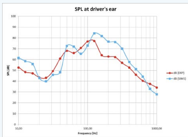
Figure 7: Sound pressure level at driver's ear compared with measured data
