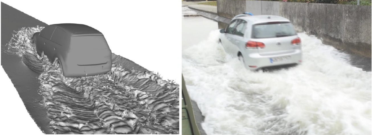
Figure 1: Comparison of FPM simulation and experimental results
