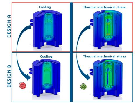
To achieve effective cooling performance, different caliber channels or routing options may be necessary. However, these changes can impact the structural compliance of the mold and vice versa.
