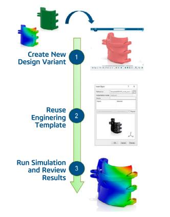
When dealing with changes in the input component, simulation templates accelerate design evaluations with minimal manual intervention. This supports faster, informed decision-making, boosting productivity.
