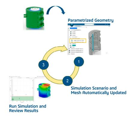
Parameterization provides designers with increased flexibility. In the platform environment, designers can adjust design parameters on the fly and automatically update all settings for previous simulation scenarios. This enables the use of parametric design studies, such as Design of Experiment, to expedite informed decision-making.
