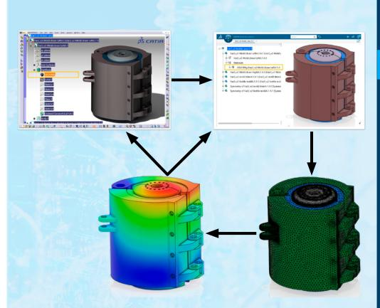
The CATIA V5 model's material data can be brought into the **3D**EXPERIENCE platform, using Power'By, and used for simulations or weight assessments. This simplified process cuts down on engineering time and supports ongoing product enhancements.
