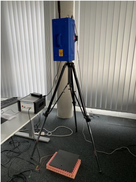
Figure 1: LDV experimental setup
