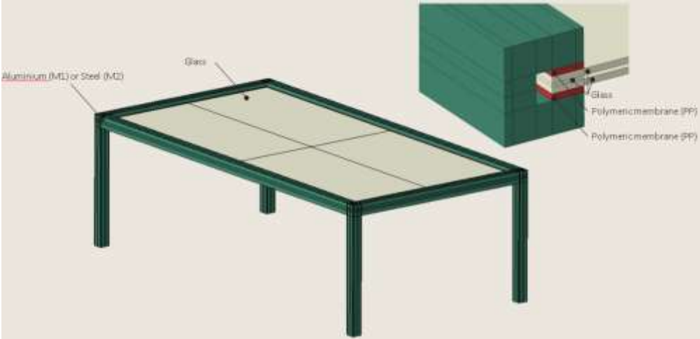
Figure 1: Glass table geometry and the materials applied to different parts
