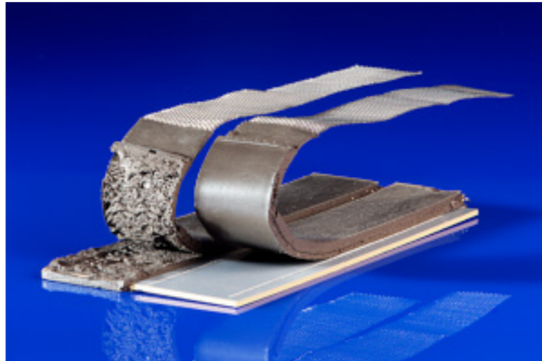
Figure 1 – Illustration of a structural adhesive joint, showcasing the complexity and diversity of materials and bonding characteristics in such connections. © Fraunhofer IFAM
