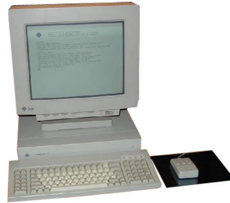
In 1993 my first real-world CFD calculations were performed using STAR-CD v2.1 on a SUN Sparc Workstation (called cfd01). I talked to the simulations using the keyboard. Note how rudimentary an early 1990s computer mouse was (Image courtesy of the PC Museum website).
