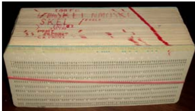
A computer program written on punched cards and wrapped with a compulsory rubber band (courtesy of ArnoldReinhold – Own work, CC BY-SA 3.0 )
