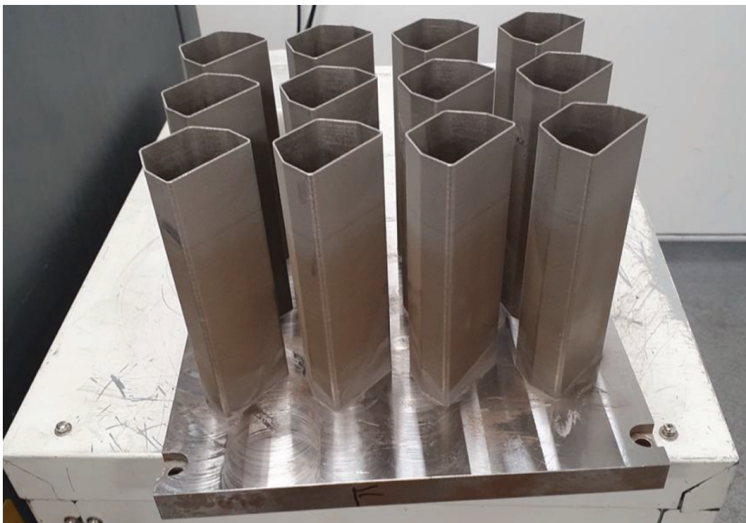
Figure 1: Twelve steel specimens that have been built at TWI with an EOS M290 (400W) machine.
