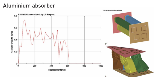
Figure 11: Axial load diagram and deformed configuration of aluminium welded energy absorber under in line impact at 36km/h with weld defects as for CASE 2.
