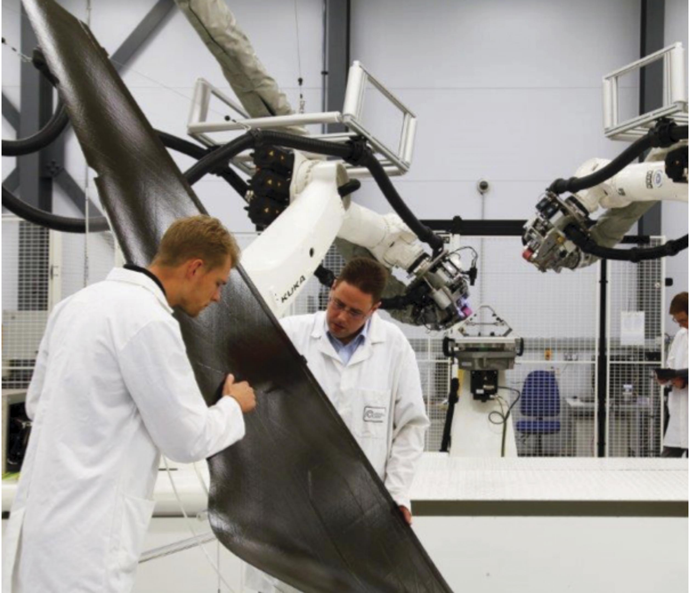
Figure 1: The NCC has two Coriolis Composites AFP machines (pictured with GKN composite winglet) and an additional Accudyne machine with choice of laser, infrared and patented Xenon FlashLamp heat sources.
