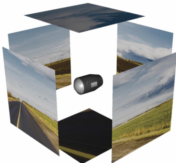
Figure 3: Six images forming a cube with a camera placed in the center
