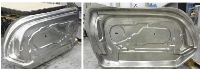
Figure 4: Industrial case, Door Inner panel provided by Lotus Cars, as successfully HFQed using Al-6082 alloy.
