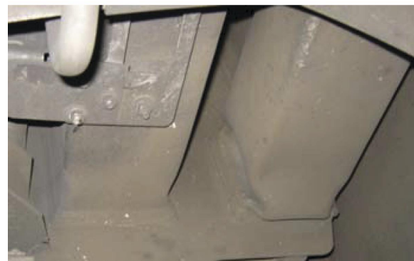
Figure 6: Energy absorbing tubes shown in situ in a rail vehicle, starter fold is clearly
