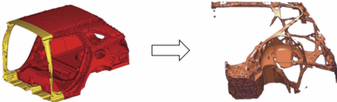
Figure 2: Linear topology optimisation: design space and remaining loadpaths [2].
