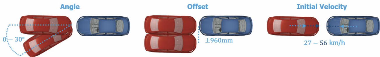
Figure 4: Crash configuration parameters and their ranges.
