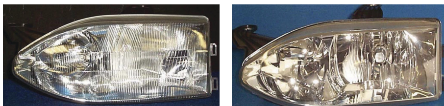
Figure 1: Comparison Between an Old Fashioned Glass Headlamp (top) and a New Transparent Plastic Headlamp (bottom)
